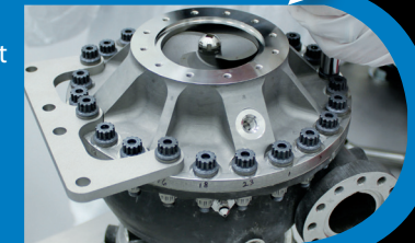
THIS ROCKET ENGINE FUEL PUMP WAS MADE BY A 3-D PRINTER!
